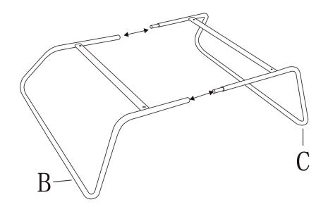
STEP 2: Attach Legs (B) (C) to Seat (A) with Spacers (E) and Bolts (D) using Allen Key (F).
